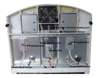
c. Open the cover of paraffin flow out lip, to replace the heating sensor and the electromagnetic valve.
