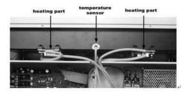
b. Open the soleplate, to replace left box, right box, platform heating parts, temperature
